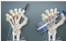
Figure 1: 3D-printed a robotic hand (ETH Zurich)
